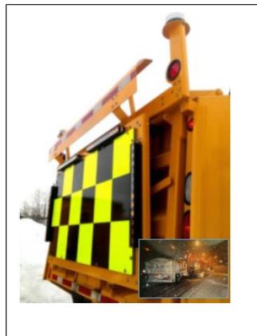
An air foil above the checkerboard panel is designed to divert air flow downwards across the panel and LED lights to reduce snow and salt accumulation.
